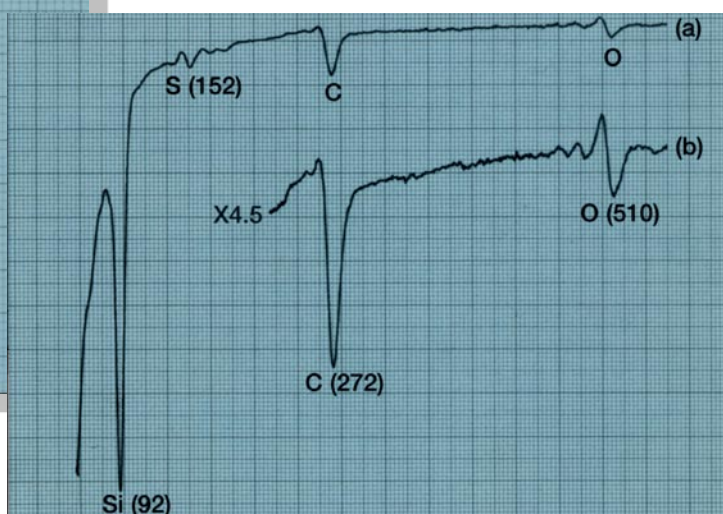
RVL2000 Auger spectra of contaminated silicon surface showing sulfur, carbon and oxygen impurities.
