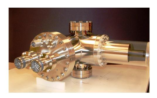
The LK1000M is an electron source of excellent energy resolution optimized for high output current. Application to inverse UPS, EELS and other electron impact experiments.
